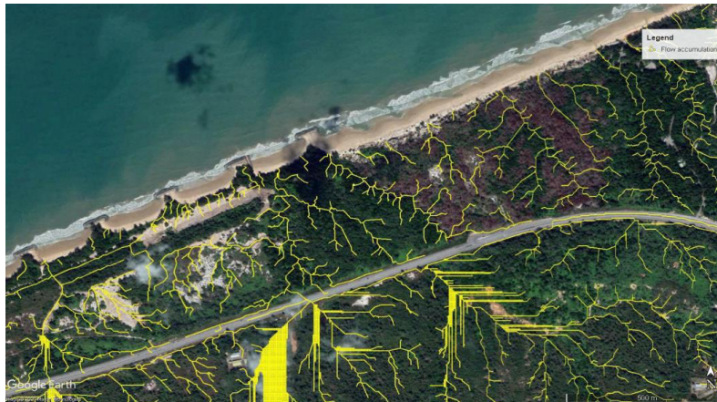
Figure 8. Gully Networks Derived from LiDAR Image Superimposed on Google Image.
